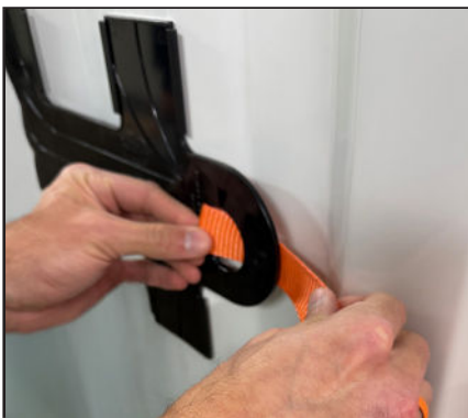
Place the banding against the container wall and slide through the handle opening.
